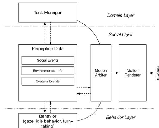
Figure 2 Block diagram for behavior generator
